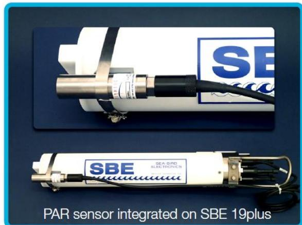
PAR sensor integrated on SBE 19plus
